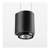
Suspended luminaire with LED, rated life of the LED L80/B10 > 50000 h, chromaticity tolerance 2 SDCM (initial), , reflector with circular light distribution pattern, reflector pure aluminium 99,99% in MIRO-Silver®, segmented and faceted, exchangeable reflector unit in high-sheen black plastic, with glass cover, luminaire housing die-cast aluminium, powder-coated, stratoblack, separate driver unit
