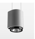
Suspended luminaire with LED, rated life of the LED L80/B10 > 50000 h, colour rendering index CRI > 80, chromaticity tolerance 2 SDCM (initial), , reflector with circular light distribution pattern, reflector pure aluminium 99,99% in MIRO-Silver®, segmented and faceted, exchangeable reflector unit in high-sheen black plastic, with glass cover, luminaire housing die-cast aluminium, powder-coated, stratosilver
