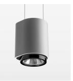
Suspended luminaire with LED, rated life of the LED L80/B10 > 50000 h, chromaticity tolerance 2 SDCM (initial), , reflector with circular light distribution pattern, reflector pure aluminium 99,99% in MIRO-Silver®, segmented and faceted, exchangeable reflector unit in high-sheen black plastic, with glass cover, luminaire housing die-cast aluminium, powder-coated, stratosilver
