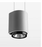
Suspended luminaire with LED, rated life of the LED L80/B10 > 50000 h, colour rendering index CRI > 90, chromaticity tolerance 2 SDCM (initial), , reflector with circular light distribution pattern, reflector pure aluminium 99,99% in MIRO-Silver®, segmented and faceted, exchangeable reflector unit in high-sheen black plastic, with glass cover, luminaire housing die-cast aluminium, powder-coated, stratosilver, separate driver unit
