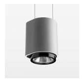
Suspended luminaire with LED, rated life of the LED L80/B10 > 50000 h, chromaticity tolerance 2 SDCM (initial), , reflector with circular light distribution pattern, reflector pure aluminium 99,99% in MIRO-Silver®, segmented and faceted, exchangeable reflector unit in high-sheen black plastic, with glass cover, luminaire housing die-cast aluminium, powder-coated, stratosilver, separate driver unit
