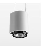
Suspended luminaire with LED, rated life of the LED L80/B10 > 50000 h, colour rendering index CRI > 80, chromaticity tolerance 2 SDCM (initial), , reflector with circular light distribution pattern, reflector pure aluminium 99,99% in MIRO-Silver®, segmented and faceted, exchangeable reflector unit in high-sheen black plastic, with glass cover, luminaire housing die-cast aluminium, powder-coated, stratowhite
