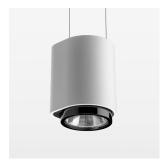
Suspended luminaire with LED, rated life of the LED L80/B10 > 50000 h, chromaticity tolerance 2 SDCM (initial), , reflector with circular light distribution pattern, reflector pure aluminium 99,99% in MIRO-Silver®, segmented and faceted, exchangeable reflector unit in high-sheen black plastic, with glass cover, luminaire housing die-cast aluminium, powder-coated, stratowhite
