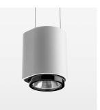
Suspended luminaire with LED, rated life of the LED L80/B10 > 50000 h, colour rendering index CRI > 96, chromaticity tolerance 3 SDCM (initial), , reflector with circular light distribution pattern, reflector pure aluminium 99,99% in MIRO-Silver®, segmented and faceted, exchangeable reflector unit in high-sheen black plastic, with glass cover, luminaire housing die-cast aluminium, powder-coated, stratowhite
