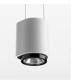
Suspended luminaire with LED, rated life of the LED L80/B10 > 50000 h, colour rendering index CRI > 90, chromaticity tolerance 2 SDCM (initial), , reflector with circular light distribution pattern, reflector pure aluminium 99,99% in MIRO-Silver®, segmented and faceted, exchangeable reflector unit in high-sheen black plastic, with glass cover, luminaire housing die-cast aluminium, powder-coated, stratowhite, separate driver unit
