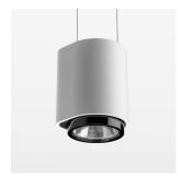
Suspended luminaire with LED, rated life of the LED L80/B10 > 50000 h, chromaticity tolerance 2 SDCM (initial), , reflector with circular light distribution pattern, reflector pure aluminium 99,99% in MIRO-Silver®, segmented and faceted, exchangeable reflector unit in high-sheen black plastic, with glass cover, luminaire housing die-cast aluminium, powder-coated, stratowhite, separate driver unit
