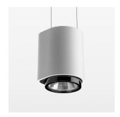
Suspended luminaire with LED, rated life of the LED L80/B10 > 50000 h, chromaticity tolerance 3 SDCM (initial), , reflector with circular light distribution pattern, reflector pure aluminium 99,99% in MIRO-Silver®, segmented and faceted, exchangeable reflector unit in high-sheen black plastic, with glass cover, luminaire housing die-cast aluminium, powder-coated, stratowhite, separate driver unit
