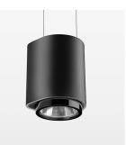
Suspended luminaire with LED, rated life of the LED L80/B10 > 50000 h, colour rendering index CRI > 80, chromaticity tolerance 2 SDCM (initial), LED hybrid technology, 3D silicone lens to reduce the proportion of scattered light, reflector with oval light distribution pattern, reflector pure aluminium 99,99% in MIRO-Silver®, segmented, exchangeable reflector unit in high-sheen black plastic, with glass cover, luminaire housing die-cast aluminium, powder-coated, stratoblack, separate driver unit
