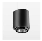
Suspended luminaire with LED, rated life of the LED L80/B10 > 50000 h, colour rendering index CRI > 80, chromaticity tolerance 2 SDCM (initial), LED hybrid technology, 3D silicone lens to reduce the proportion of scattered light, reflector with oval light distribution pattern, reflector pure aluminium 99,99% in MIRO-Silver®, segmented, exchangeable reflector unit in high-sheen black plastic, with glass cover, luminaire housing die-cast aluminium, powder-coated, stratoblack
