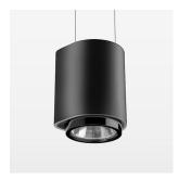
Suspended luminaire with LED, rated life of the LED L80/B10 > 50000 h, chromaticity tolerance 2 SDCM (initial), LED hybrid technology, 3D silicone lens to reduce the proportion of scattered light, reflector with oval light distribution pattern, reflector pure aluminium 99,99% in MIRO-Silver®, segmented, exchangeable reflector unit in high-sheen black plastic, with glass cover, luminaire housing die-cast aluminium, powder-coated, stratoblack
