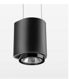
Suspended luminaire with LED, rated life of the LED L80/B10 > 50000 h, colour rendering index CRI > 96, chromaticity tolerance 3 SDCM (initial), LED hybrid technology, 3D silicone lens to reduce the proportion of scattered light, reflector with oval light distribution pattern, reflector pure aluminium 99,99% in MIRO-Silver®, segmented, exchangeable reflector unit in high-sheen black plastic, with glass cover, luminaire housing die-cast aluminium, powder-coated, stratoblack
