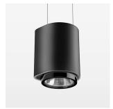
Suspended luminaire with LED, rated life of the LED L80/B10 > 50000 h, chromaticity tolerance 2 SDCM (initial), LED hybrid technology, 3D silicone lens to reduce the proportion of scattered light, reflector with oval light distribution pattern, reflector pure aluminium 99,99% in MIRO-Silver®, segmented, exchangeable reflector unit in high-sheen black plastic, with glass cover, luminaire housing die-cast aluminium, powder-coated, stratoblack
