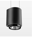
Suspended luminaire with LED, rated life of the LED L80/B10 > 50000 h, chromaticity tolerance 2 SDCM (initial), LED hybrid technology, 3D silicone lens to reduce the proportion of scattered light, reflector with oval light distribution pattern, reflector pure aluminium 99,99% in MIRO-Silver®, segmented, exchangeable reflector unit in high-sheen black plastic, with glass cover, luminaire housing die-cast aluminium, powder-coated, stratoblack, separate driver unit
