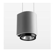
Suspended luminaire with LED, rated life of the LED L80/B10 > 50000 h, colour rendering index CRI > 80, chromaticity tolerance 2 SDCM (initial), LED hybrid technology, 3D silicone lens to reduce the proportion of scattered light, reflector with oval light distribution pattern, reflector pure aluminium 99,99% in MIRO-Silver®, segmented, exchangeable reflector unit in highsheen black plastic, with glass cover, luminaire housing die-cast aluminium, powder-coated, stratosilver, separate driver unit
