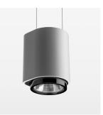
Suspended luminaire with LED, rated life of the LED L80/B10 > 50000 h, colour rendering index CRI > 90, chromaticity tolerance 2 SDCM (initial), LED hybrid technology, 3D silicone lens to reduce the proportion of scattered light, reflector with oval light distribution pattern, reflector pure aluminium 99,99% in MIRO-Silver®, segmented, exchangeable reflector unit in high-sheen black plastic, with glass cover, luminaire housing die-cast aluminium, powder-coated, stratosilver, separate driver unit
