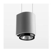
Suspended luminaire with LED, rated life of the LED L80/B10 > 50000 h, colour rendering index CRI > 90, chromaticity tolerance 2 SDCM (initial), LED hybrid technology, 3D silicone lens to reduce the proportion of scattered light, reflector with oval light distribution pattern, reflector pure aluminium 99,99% in MIRO-Silver®, segmented, exchangeable reflector unit in high-sheen black plastic, with glass cover, luminaire housing die-cast aluminium, powder-coated, stratosilver, separate driver unit
