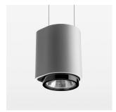
Suspended luminaire with LED, rated life of the LED L80/B10 > 50000 h, chromaticity tolerance 2 SDCM (initial), LED hybrid technology, 3D silicone lens to reduce the proportion of scattered light, reflector with oval light distribution pattern, reflector pure aluminium 99,99% in MIRO-Silver®, segmented, exchangeable reflector unit in high-sheen black plastic, with glass cover, luminaire housing die-cast aluminium, powder-coated, stratosilver
