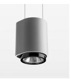
Suspended luminaire with LED, rated life of the LED L80/B10 > 50000 h, colour rendering index CRI > 96, chromaticity tolerance 3 SDCM (initial), LED hybrid technology, 3D silicone lens to reduce the proportion of scattered light, reflector with oval light distribution pattern, reflector pure aluminium 99,99% in MIRO-Silver®, segmented, exchangeable reflector unit in high-sheen black plastic, with glass cover, luminaire housing die-cast aluminium, powder-coated, stratosilver
