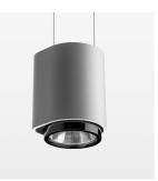
Suspended luminaire with LED, rated life of the LED L80/B10 > 50000 h, chromaticity tolerance 3 SDCM (initial), LED hybrid technology, 3D silicone lens to reduce the proportion of scattered light, reflector with oval light distribution pattern, reflector pure aluminium 99,99% in MIRO-Silver®, segmented, exchangeable reflector unit in high-sheen black plastic, with glass cover, luminaire housing die-cast aluminium, powder-coated, stratosilver, separate driver unit
