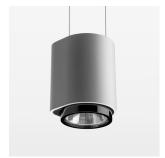
Suspended luminaire with LED, rated life of the LED L80/B10 > 50000 h, chromaticity tolerance 3 SDCM (initial), LED hybrid technology, 3D silicone lens to reduce the proportion of scattered light, reflector with oval light distribution pattern, reflector pure aluminium 99,99% in MIRO-Silver®, segmented, exchangeable reflector unit in high-sheen black plastic, with glass cover, luminaire housing die-cast aluminium, powder-coated, stratosilver, separate driver unit
