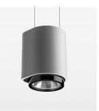
Suspended luminaire with LED, rated life of the LED L80/B10 > 50000 h, chromaticity tolerance 2 SDCM (initial), LED hybrid technology, 3D silicone lens to reduce the proportion of scattered light, reflector with oval light distribution pattern, reflector pure aluminium 99,99% in MIRO-Silver®, segmented, exchangeable reflector unit in high-sheen black plastic, with glass cover, luminaire housing die-cast aluminium, powder-coated, stratosilver, separate driver unit
