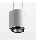
Suspended luminaire with LED, rated life of the LED L80/B10 > 50000 h, colour rendering index CRI > 90, chromaticity tolerance 2 SDCM (initial), LED hybrid technology, 3D silicone lens to reduce the proportion of scattered light, reflector with oval light distribution pattern, reflector pure aluminium 99,99% in MIRO-Silver®, segmented, exchangeable reflector unit in high-sheen black plastic, with glass cover, luminaire housing die-cast aluminium, powder-coated, stratowhite, separate driver unit
