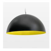
Decorative suspended luminaire with hub holder E27, max 150W, shade made of painted aluminium, black / traffic yellow, metal trim ring (diameter 95mm) around hub holder, 28 ventilation openings (diameter 5mm) conzentric circular arrangement, double-isulated cabling, clampingdevice on cable ends if feed cable > 80 mm, power feed cable and canopy black, steel cable hanging set, ceiling-mounting, 1.5m cable
