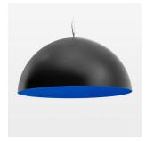
Decorative suspended luminaire with hub holder E27, max 150W, shade made of painted aluminium, black / traffic blue, metal trim ring (diameter 95mm) around hub holder, 28 ventilation openings (diameter 5mm) conzentric circular arrangement, double-isulated cabling, clampingdevice on cable ends if feed cable > 80 mm, power feed cable and canopy black, steel cable hanging set, ceiling-mounting, 3m cable
