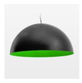
Decorative suspended luminaire with hub holder E27, max 150W, shade made of painted aluminium, black / yellow-green, metal trim ring (diameter 95mm) around hub holder, 28 ventilation openings (diameter 5mm) conzentric circular arrangement, double-isulated cabling, clampingdevice on cable ends if feed cable > 80 mm, power feed cable and canopy black, steel cable hanging set, ceiling-mounting, 6m cable
