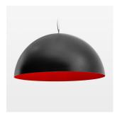
Decorative suspended luminaire with hub holder E27, max 150W, shade made of painted aluminium, black / traffic red, metal trim ring (diameter 95mm) around hub holder, 28 ventilation openings (diameter 5mm) conzentric circular arrangement, double-isulated cabling, clampingdevice on cable ends if feed cable > 80 mm, power feed cable and canopy black, steel cable hanging set, ceiling-mounting, 6m cable
