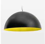
Decorative suspended luminaire with hub holder E27, max 150W, shade made of painted aluminium, black / traffic yellow, metal trim ring (diameter 95mm) around hub holder, 28 ventilation openings (diameter 5mm) conzentric circular arrangement, double-isulated cabling, clampingdevice on cable ends if feed cable > 80 mm, power feed cable and canopy black, steel cable hanging set, multiadapter, 1.5m cable
