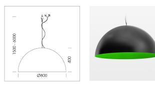
Decorative suspended luminaire with hub holder E27, max 150W, shade made of painted aluminium, black / yellow-green, metal trim ring (diameter 95mm) around hub holder, 28 ventilation openings (diameter 5mm) conzentric circular arrangement, double-isulated cabling, clampingdevice on cable ends if feed cable > 80 mm, power feed cable and canopy black, steel cable hanging set, multiadapter, 1.5m cable
