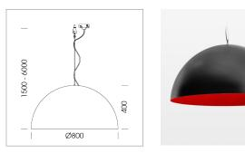
Decorative suspended luminaire with hub holder E27, max 150W, shade made of painted aluminium, black / traffic red, metal trim ring (diameter 95mm) around hub holder, 28 ventilation openings (diameter 5mm) conzentric circular arrangement, double-isulated cabling, clampingdevice on cable ends if feed cable > 80 mm, power feed cable and canopy black, steel cable hanging set, multiadapter, 1.5m cable
