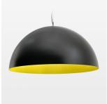
Decorative suspended luminaire with hub holder E27, max 150W, shade made of painted aluminium, black / traffic yellow, metal trim ring (diameter 95mm) around hub holder, 28 ventilation openings (diameter 5mm) conzentric circular arrangement, double-isulated cabling, clampingdevice on cable ends if feed cable > 80 mm, power feed cable and canopy black, steel cable hanging set, multiadapter, 3m cable
