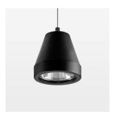
Suspended luminaire with LED, rated life of the LED L80/B10 > 50000 h, colour rendering index CRI > 80, chromaticity tolerance 3 SDCM (initial), rotation-symmetrical reflector with circular light distribution pattern, reflector pure aluminium 99,99% in MIRO-Silver®, segmented and faceted, 3D lens silicon to reduce the proportion of scattered light, luminaire head die-cast aluminium, powder-coated, stratoblack
