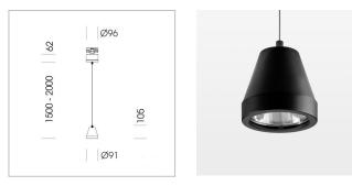
Suspended luminaire with LED, rated life of the LED L80/B10 > 50000 h, colour rendering index CRI > 90, chromaticity tolerance 3 SDCM (initial), rotation-symmetrical reflector with circular light distribution pattern, reflector pure aluminium 99,99% in MIRO-Silver®,segmented and faceted, 3D lens silicon to reduce the proportion of scattered light, luminaire head die-cast aluminium, powder-coated, stratoblack
