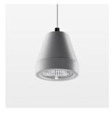
Suspended luminaire with LED, rated life of the LED L80/B10 > 50000 h, colour rendering index CRI > 96, chromaticity tolerance 2 SDCM (initial), rotation-symmetrical reflector with circular light distribution pattern, reflector pure aluminium 99,99% in MIRO-Silver®, segmented and faceted, 3D lens silicon to reduce the proportion of scattered light, luminaire head die-cast aluminium, powder-coated, stratosilver
