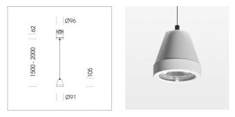
Suspended luminaire with LED, rated life of the LED L80/B10 > 50000 h, colour rendering index CRI > 80, chromaticity tolerance 3 SDCM (initial), rotation-symmetrical reflector with circular light distribution pattern, reflector pure aluminium 99,99% in MIRO-Silver®,segmented and faceted, 3D lens silicon to reduce the proportion of scattered light, luminaire head die-cast aluminium, powder-coated, stratowhite
