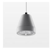
Suspended luminaire with LED, rated life of the LED L80/B10 > 50000 h, colour rendering index CRI > 90, chromaticity tolerance 2 SDCM (initial), rotation-symmetrical reflector with circular light distribution pattern, reflector pure aluminium 99,99% in MIRO-Silver®, segmented and faceted, 3D lens silicon to reduce the proportion of scattered light, luminaire head die-cast aluminium, powder-coated, stratosilver
