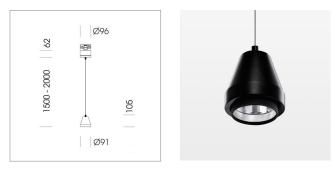
Suspended luminaire with LED, rated life of the LED L80/B10 > 50000 h, colour rendering index CRI > 96, chromaticity tolerance 3 SDCM (initial), reflector with circular light distribution pattern, reflector pure aluminium 99,99% in MIRO-Silver®,segmented and faceted, 3D lens silicon to reduce the proportion of scattered light, luminaire head die-cast aluminium, powdercoated, stratoblack
