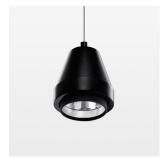
Suspended luminaire with LED, rated life of the LED L80/B10 > 50000 h, colour rendering index CRI > 90, chromaticity tolerance 2 SDCM (initial), reflector with circular light distribution pattern, reflector pure aluminium 99,99% in MIRO-Silver®, segmented and faceted, 3D lens silicon to reduce the proportion of scattered light, luminaire head die-cast aluminium, powder-coated, stratoblack
