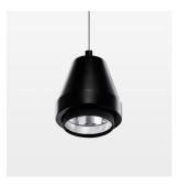
Suspended luminaire with LED, rated life of the LED L80/B10 > 50000 h, chromaticity tolerance 2 SDCM (initial), reflector with circular light distribution pattern, reflector pure aluminium 99,99% in MIRO-Silver®,segmented and faceted, 3D lens silicon to reduce the proportion of scattered light, luminaire head die-cast aluminium, powder-coated, stratoblack
