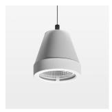
Suspended luminaire with LED, rated life of the LED L80/B10 > 50000 h, colour rendering index CRI > 96, chromaticity tolerance 3 SDCM (initial), reflector with circular light distribution pattern, reflector pure aluminium 99,99% in MIRO-Silver®, segmented and faceted, 3D lens silicon to reduce the proportion of scattered light, luminaire head die-cast aluminium, powder-coated, stratowhite
