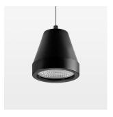
Suspended luminaire with LED, rated life of the LED L80/B10 > 50000 h, colour rendering index CRI > 80, chromaticity tolerance 2 SDCM (initial), reflector with circular light distribution pattern, reflector pure aluminium 99,99% in MIRO-Silver®, segmented and faceted, luminaire head die-cast aluminium, powder-coated, stratoblack
