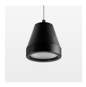
Suspended luminaire with LED, rated life of the LED L80/B10 > 50000 h, chromaticity tolerance 2 SDCM (initial), reflector with circular light distribution pattern, reflector pure aluminium 99,99% in MIRO-Silver®,segmented and faceted, luminaire head die-cast aluminium, powder-coated, stratoblack
