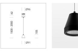
Suspended luminaire with LED, rated life of the LED L80/B10 > 50000 h, colour rendering index CRI > 96, chromaticity tolerance 3 SDCM (initial), reflector with circular light distribution pattern, reflector pure aluminium 99,99% in MIRO-Silver®,segmented and faceted, luminaire head die-cast aluminium, powder-coated, stratoblack
