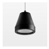
Suspended luminaire with LED, rated life of the LED L80/B10 > 50000 h, colour rendering index CRI > 96, chromaticity tolerance 3 SDCM (initial), reflector with circular light distribution pattern, reflector pure aluminium 99,99% in MIRO-Silver®, segmented and faceted, luminaire head die-cast aluminium, powder-coated, stratoblack
