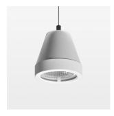
Suspended luminaire with LED, rated life of the LED L80/B10 > 50000 h, colour rendering index CRI > 96, chromaticity tolerance 3 SDCM (initial), reflector with circular light distribution pattern, reflector pure aluminium 99,99% in MIRO-Silver®, segmented and faceted, luminaire head die-cast aluminium, powder-coated, stratowhite
