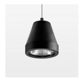
Suspended luminaire with LED, rated life of the LED L80/B10 > 50000 h, colour rendering index CRI > 95, chromaticity tolerance 2 SDCM (initial), rotation-symmetrical reflector with circular light distribution pattern, reflector pure aluminium 99,99% in MIRO-Silver®, segmented and faceted, 3D lens silicon to reduce the proportion of scattered light, luminaire head die-cast aluminium, powder-coated, stratoblack
