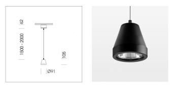
Suspended luminaire with LED, rated life of the LED L80/B10 > 50000 h, colour rendering index CRI > 96, chromaticity tolerance 2 SDCM (initial), rotation-symmetrical reflector with circular light distribution pattern, reflector pure aluminium 99,99% in MIRO-Silver®,segmented and faceted, 3D lens silicon to reduce the proportion of scattered light, luminaire head die-cast aluminium, powder-coated, stratoblack
